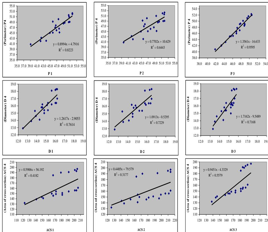
Fig 1: Relationship between measured and calculated values of fiber perimeter, diameter and area of cross section
