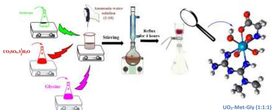
**Fig 2.** Schematic preparation of  $\text{UO}_2\text{-Met-Gly}$  complex (1:1:1)
