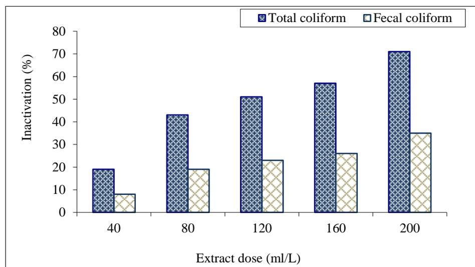
**Figure (1):** Effect of mint aqueous extract dose on total and fecal coliform within one hour.
