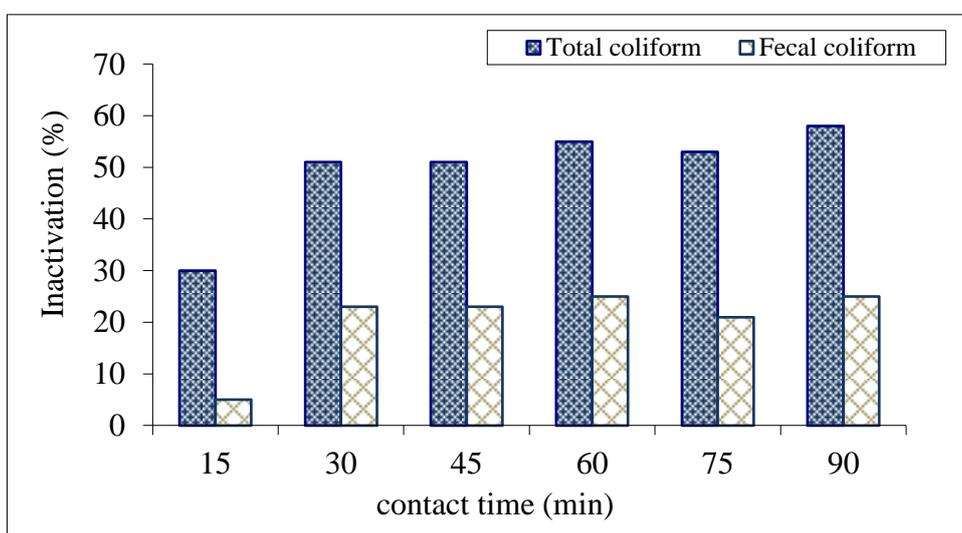
**Figure (2):** Effect of different contact time on total and fecal coliform by 40ml/l mint extract dose
