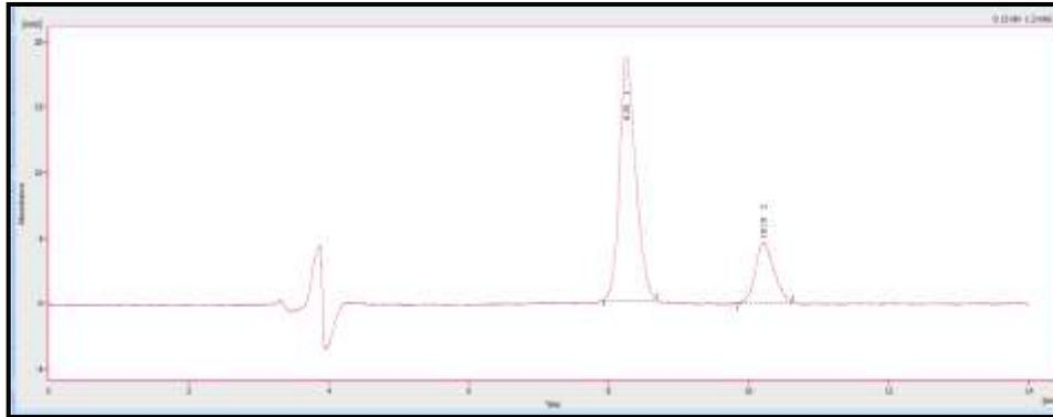
Figure 2. HPLC chromatogram of a standard mixture of 5-HMF and patulin.
