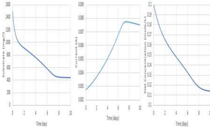
**Figure 1 Change of substrate concentration, current produced and salt concentration in desalination chamber with time**
