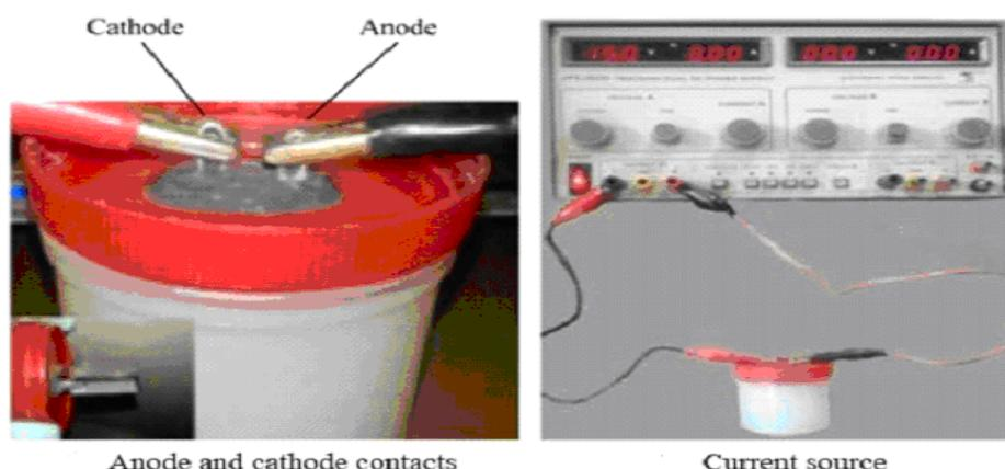
**Figure (2): Coating process with electrophoretic method**
