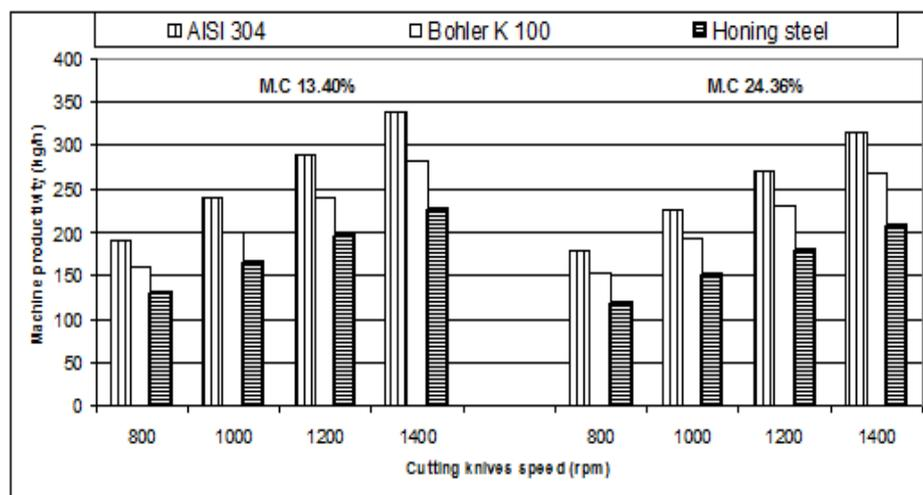
**Fig. (5). Effect of cutting-knives speed, rice-straw moisture content and alloy type on machine productivity.**
