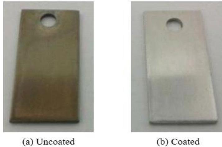
**Figure (3):** Uncoated and coated knives
