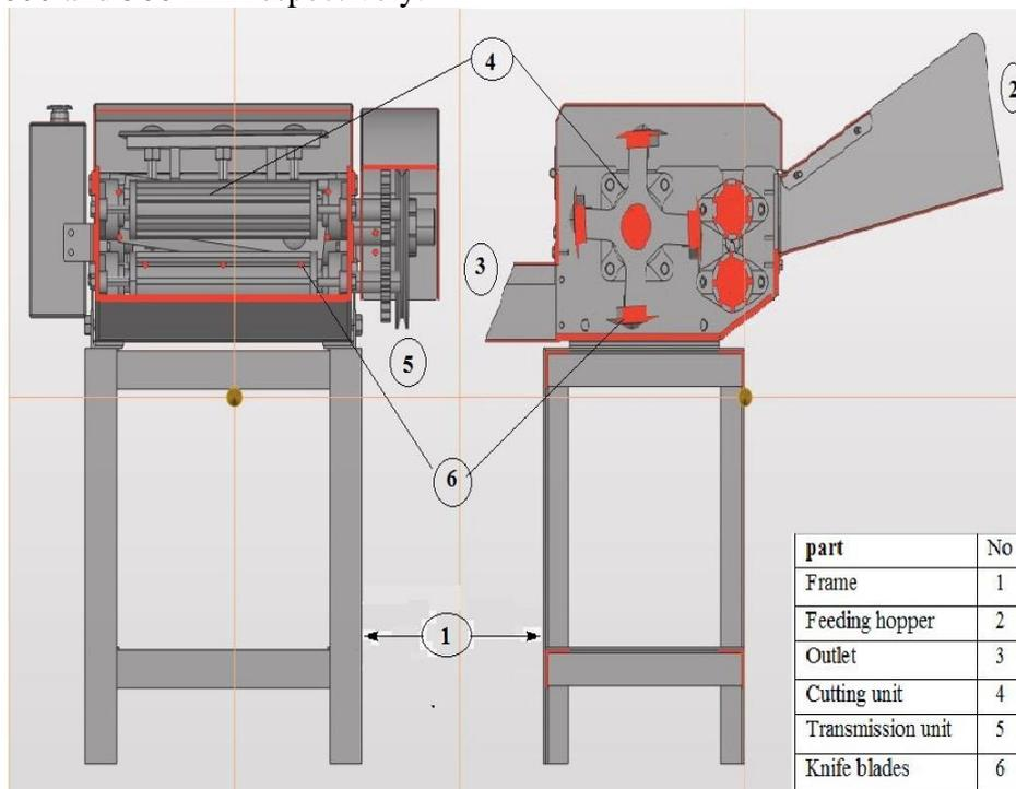
**Figure (1): Developed disc-chopper views**
