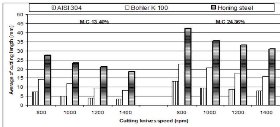
**Fig. (4). Effect of cutting-knives speed, rice-straw moisture content and alloy type on average of cutting length.**
