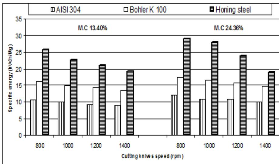
**Fig. (6). Effect of cutting-knives speed, rice-straw moisture content and alloy type on specific energy.**
