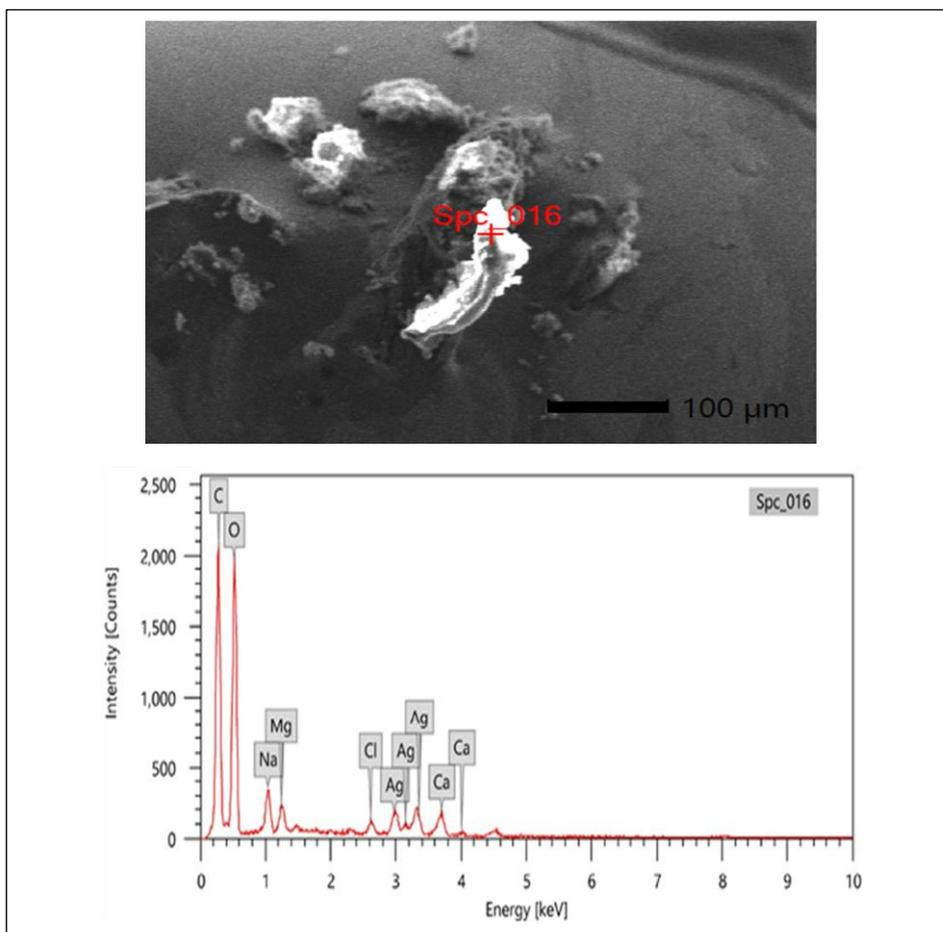
**Fig (3) . EDX analysis of biosynthesized AgNPs by Dates aqueous extract.**
