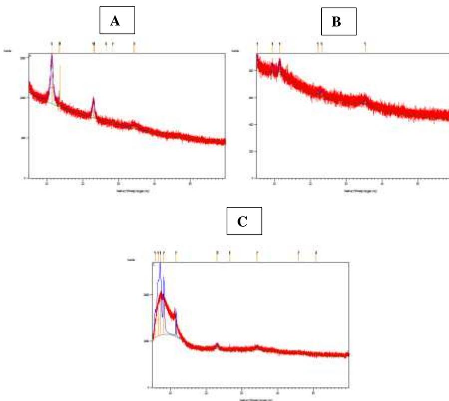
**Figure 2:** XRD charts of the LDH samples of different treatments. A: represent L. B: represent LH1. D: represent LH2.
