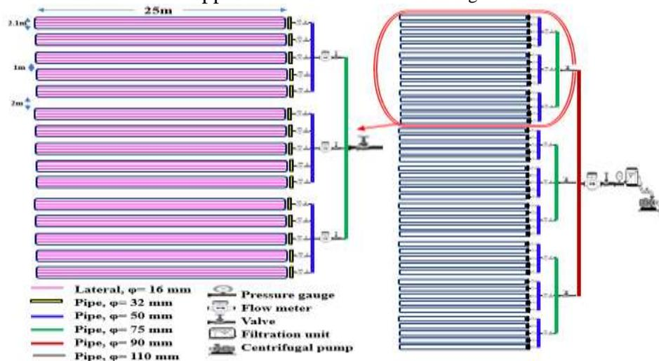
Figure 1: Drip irrigation system components.
