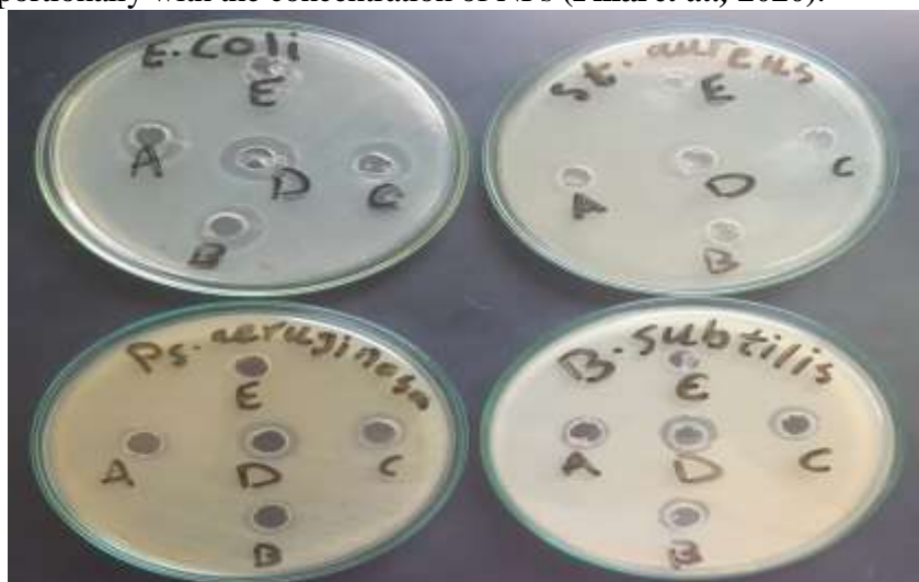
Fig 5. Antibacterial activity of biosynthesized ZnO NPs (A: 10 µg/ml, B: 25 µg/ml, C: 50 µg/ml, D: ceftriaxone 10 µg/ml, and E: distilled water).
