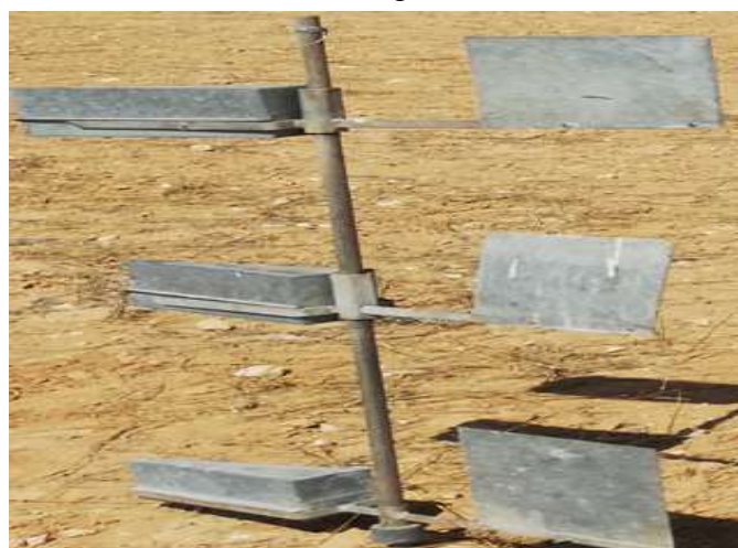
Fig (2): The Big Spring Number Eight (BSNE) trap ( Fryrear, 1986 )
