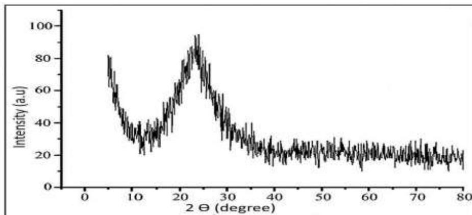
**Figure (3):** X-ray Diffraction patterns of the formed SiNPs.
