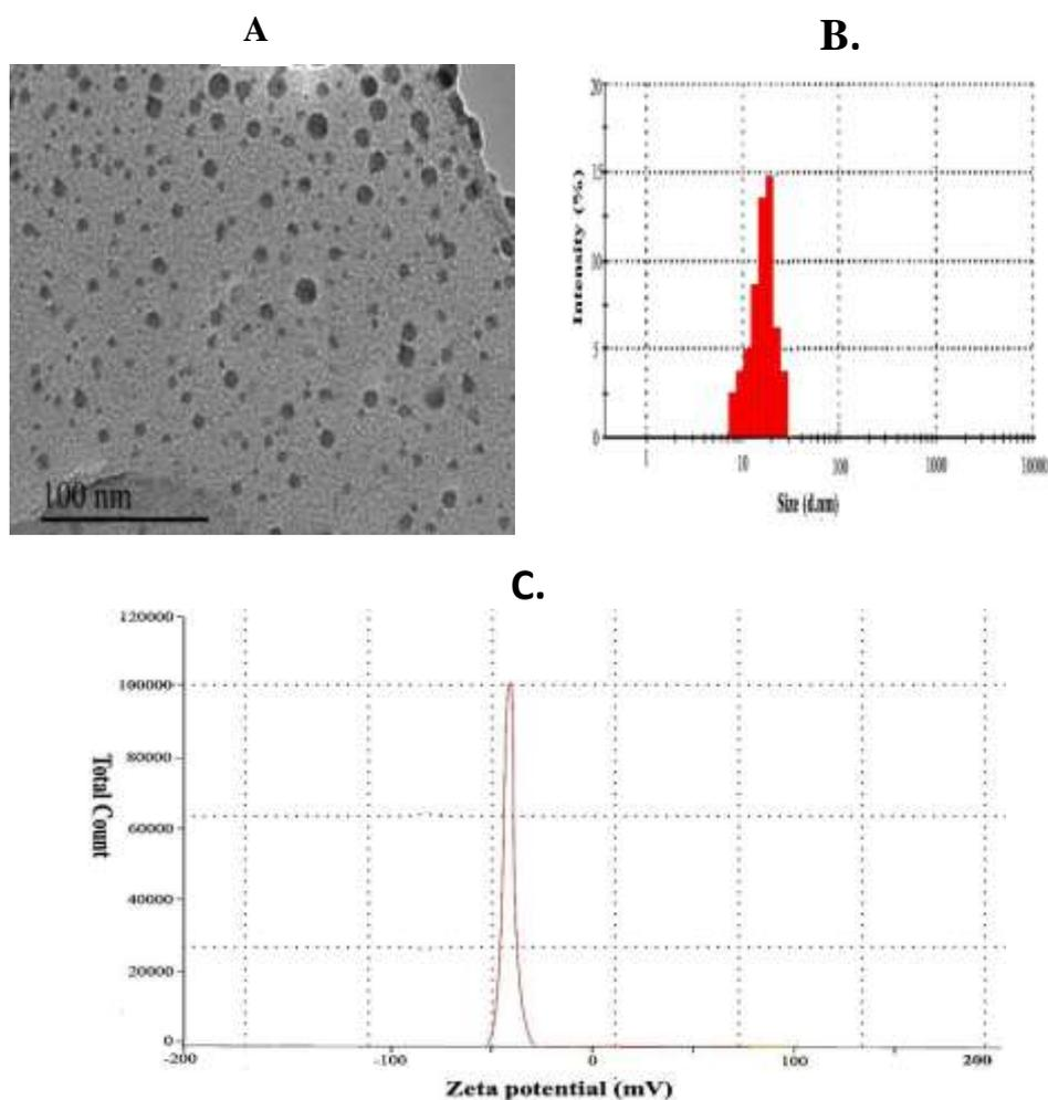
**Fig.(2):** Characterization of the formed silica nanoparticles:(A.) TEM image of the formed SiNPs, (B) & (C) the particle and the zeta potential of the formed SiNPs respectively.
