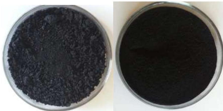
Granular Bagasse active carbon      Powder Bagasse active carbon
